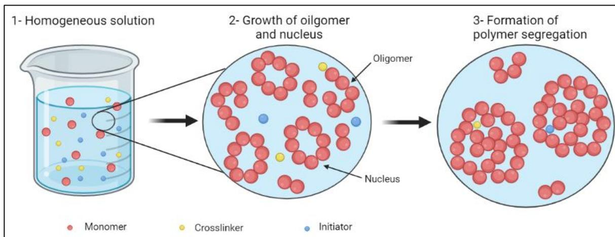
**Figure 7: Precipitation polymerization**
