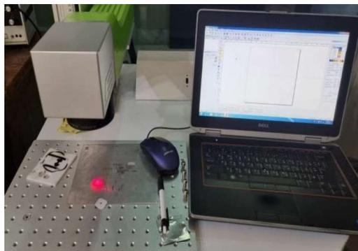
**Figure 4: Acrylic (disc shape) specimens during treatment with Nd: YAG laser**
