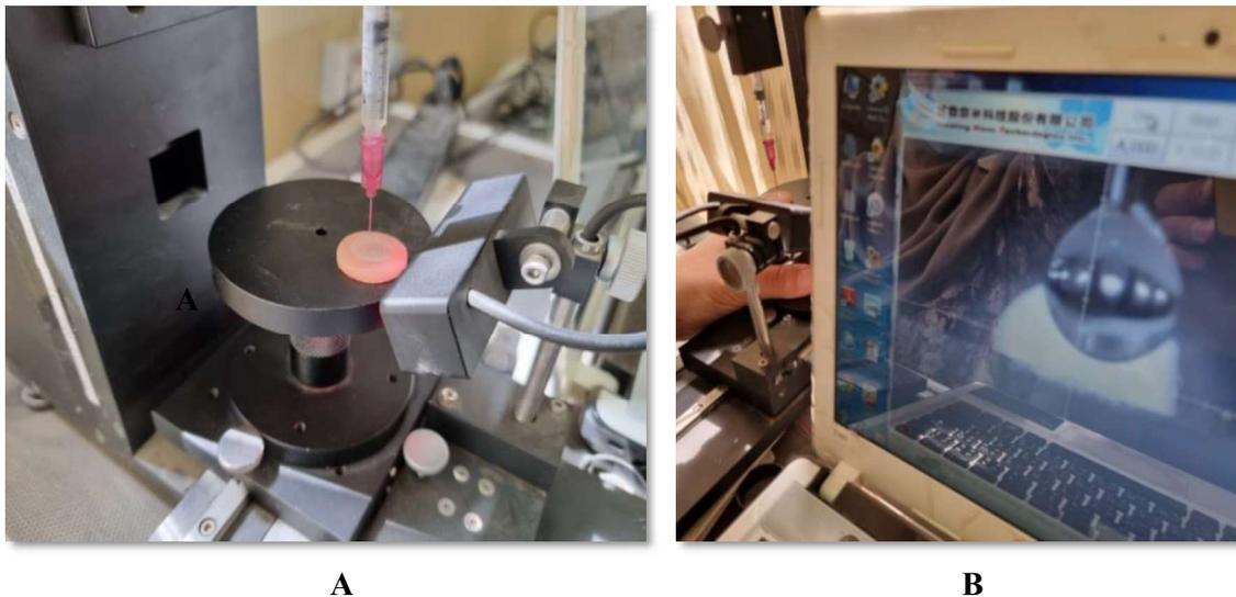
**Figure 5: (A, B): Show the wetting and surface energy characteristics of the wettability test**
