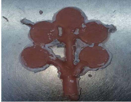
**Figure 2: disc shaped specimens of thermoplastic acrylic after deflasking**
