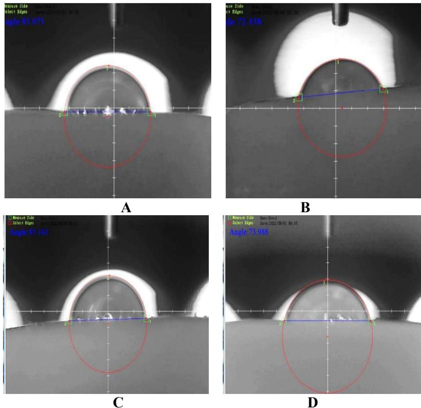
Figure 7: Digital images of goniometer measurements of contact angle; (A) group TC, (B) group TT, (C) group HC, and (D) group HT.
